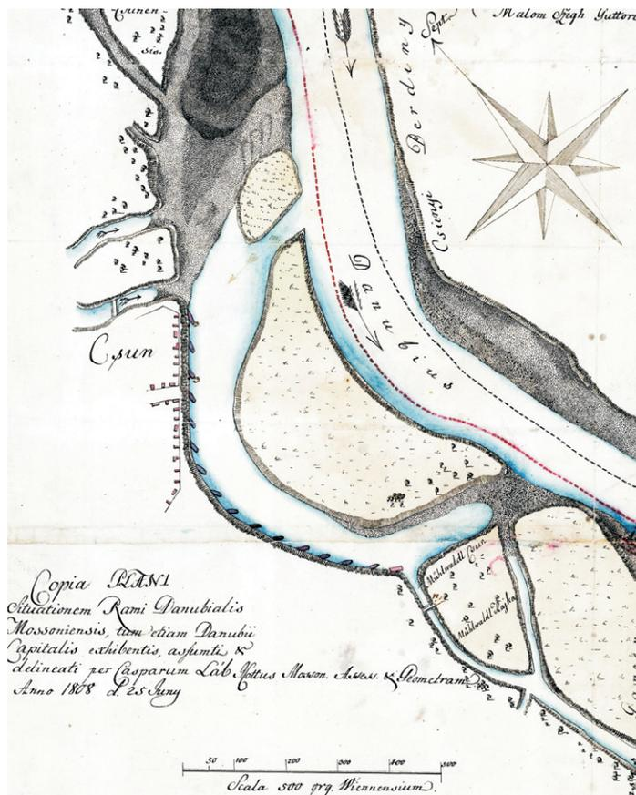
Fig. 8: The map from 25 June 1808 showing the Čunovo meander after its abandonment. Until 1796, a total of 16 stone groynes up to 40 m long were constructed to protect the Čunovo undercut banks
