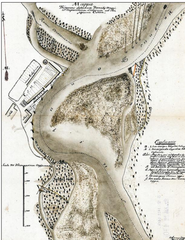
Fig. 3: Within only 6 years a brand new prominent meander of the mainchannel developed at Čunovo, partly destroying the village itself. Its rapid development is indirectly evidenced by the large unvegetated point bar. The 1790 manuscript map by Casparus Láb also shows detailed remedial measures intended to control erosion and to divert the dangerous flow
