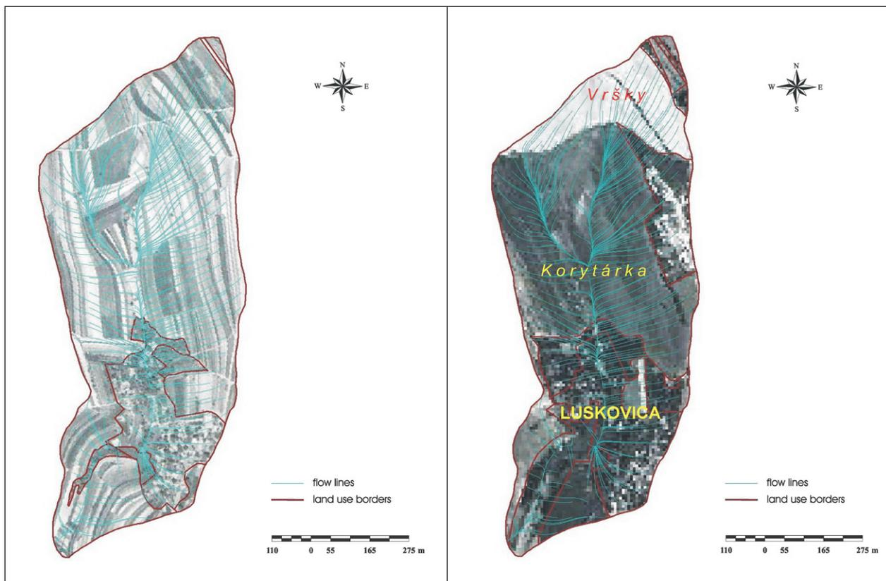
Fig. 3: Land use according to aerial photographs from 1955 (left) and 1990 with indicated flow lines constructed downhill (right)
