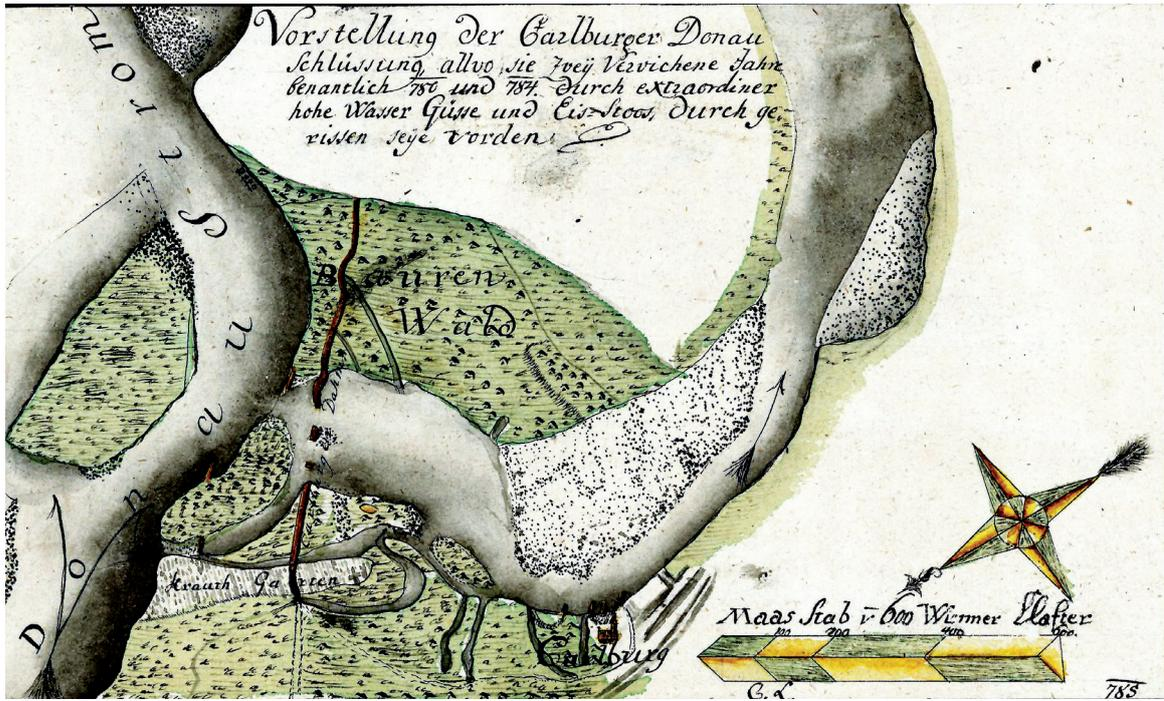
Fig. 7: Breaches to side-channel closure (and dike) at the village of Rusovce (Carlburg), illustrating the destructive force of 1780 and 1784 ice floods. Heavy lateral erosion in re-activated channel during these floods was also indirectly evidenced by extensive unvegetated point bars
