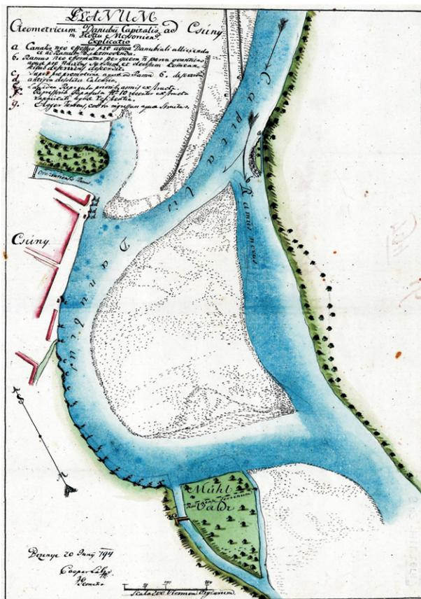
Fig. 5: The map from 20 June 1794 already shows the flow successfully deflected into a new, straighter channel. Nevertheless, heavy bank erosion was still continuing in the original bend, as well. Apart from 6 stone groynes, built in the preceding years, the map depicts additional 10 projected groynes
