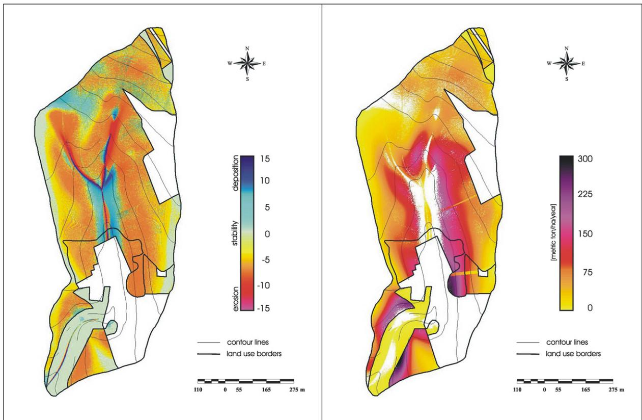
Fig. 5: Potential water erosion according to models USPED (left) and USLE for 1990 (right)
