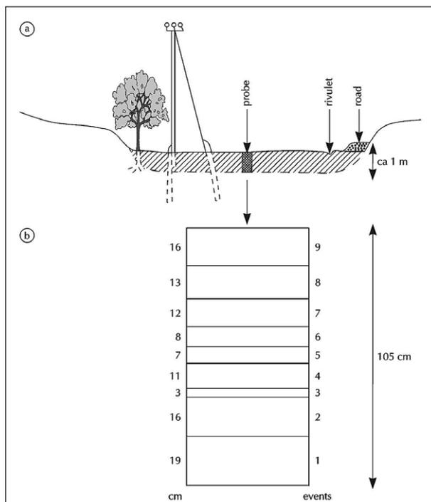
Fig. 7: Cross-profile of dry valley bottom at the hamlet of Luskovica with enlargement of test
