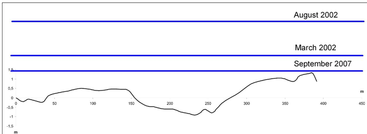
Fig. 3: Floodplain cross-section profile (for location see Fig. 2), with estimated levels of flood waters
