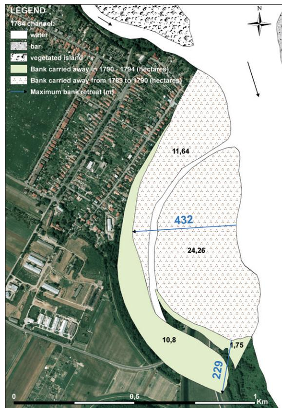
Fig. 4: Land carried away during the evolution of a new Danube bend in periods 1783–1790 and 1790–1794, respectively. Arrows designate the lines of maximum bank retreat (in metres) from which maximum bank erosion rates were derived
