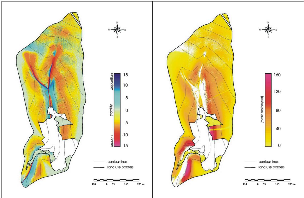
Fig. 4: Potential water erosion according to models USPED (left) and USLE for 1955 (right)
